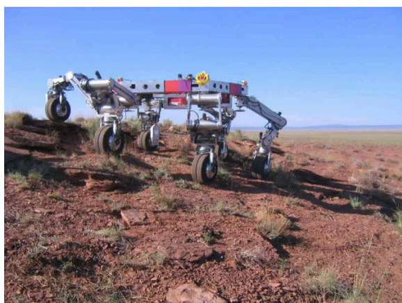
Figure 3. ATHLETE (All-Terrain Hex-Limbed Extra-Terrestrial Explorer) vehicle.
