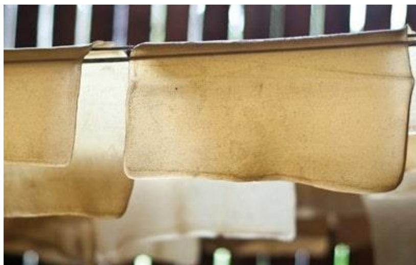
Figure 7 – Liquid Smoked Sheet drying on wires in an artisanal rubber plant
