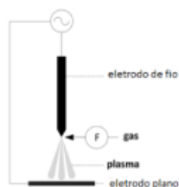
Figura 4 - Reator de plasma frio descarga corona (SUROWSKY; SCHLUÜTER; KNORR, 2014).
