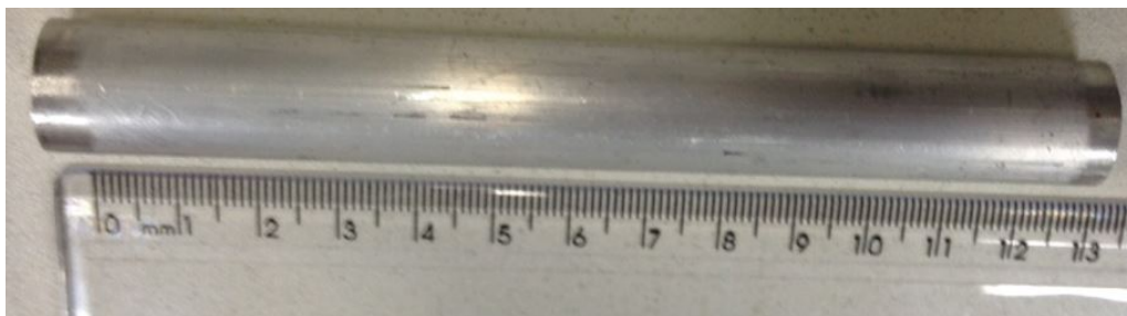
Figure 2- Cylindrical specimen before compression test.
