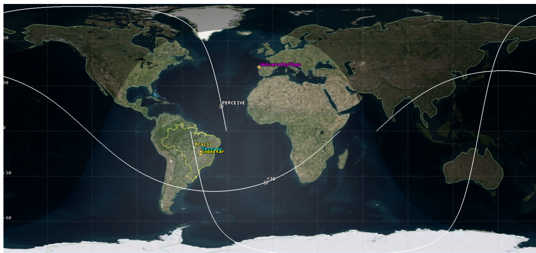
Figure 1.: Representation of the analyzed ground stations and the ground tracks of the SSO and MIO orbital configurations.
