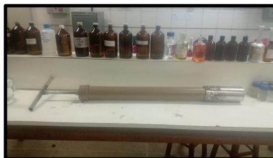
Figura 1: Coletor Core Sample
