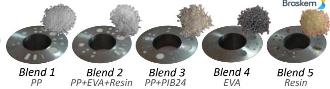
5 polymer blends were developed and infiltrated into the simplified specimen
