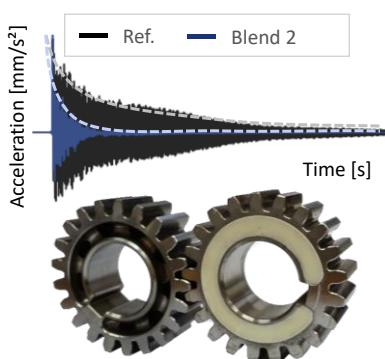
The “Blend 2” polymer was chosen to infiltrate the gear web and evaluate NVH performance
