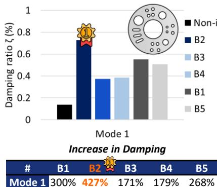
The “Blend 2” polymer showed 4 times higher damping compared to the simplified non-infiltrated specimen
