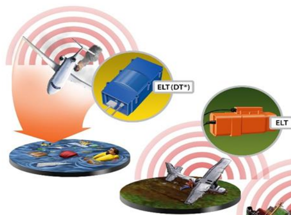
Figure 1: Activation of the ELT-DT during flight and the ELT after impact. Source: ICAO.
