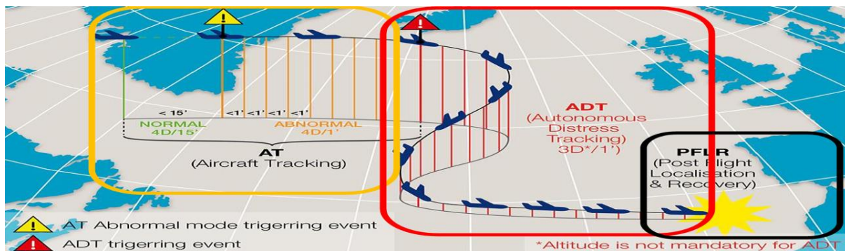
Figure 3: ELT-DT activated in flight due to abnormal aircraft behavior. Source: Eurocontrol (2020).
