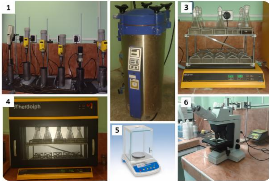
Figure 1. Equipment used: (1) Bioreactors, (2) reactor, (3) Stirrer screen, (4) Orbital screen with thermostat, (5) Analytical balance, (6) Optical microscope. Source: authors
