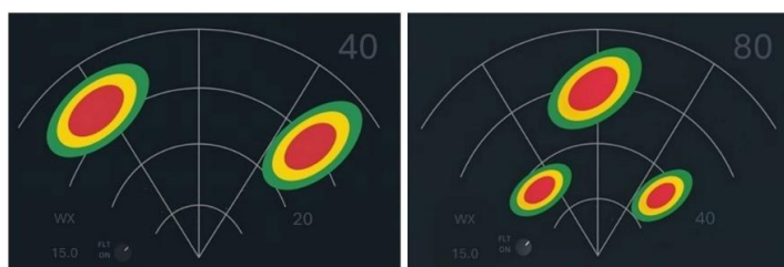
Figure 4: False corridor impression due to the use of the wrong range (on the left), in contrast to the use of a further range (on the right) for the meteorological radar.
