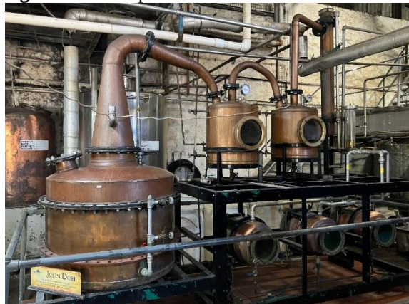
Figura 5. Alambique “double retort” Saint Lucia Distillers
